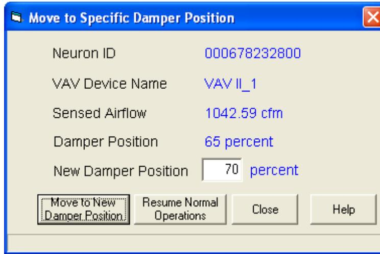
Fig. 15. Move to Damper Position.
