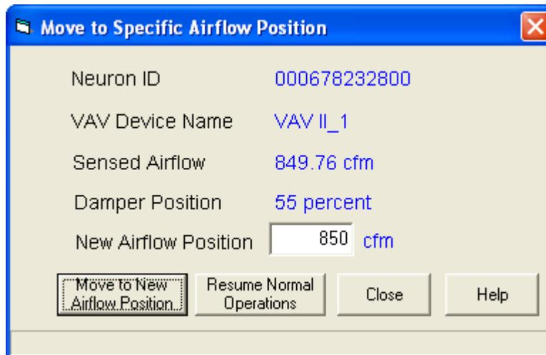
Fig. 16. Move to Airflow Position.
