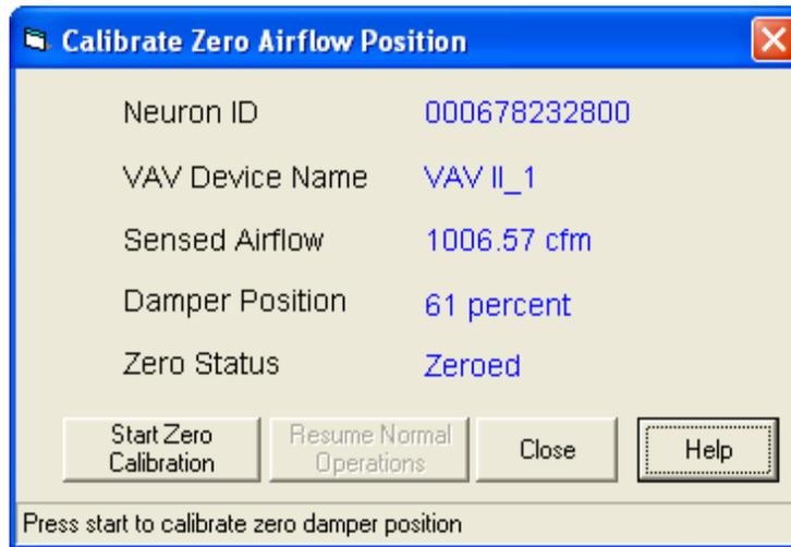
Fig. 17. Calibrate Zero Airflow Position.
