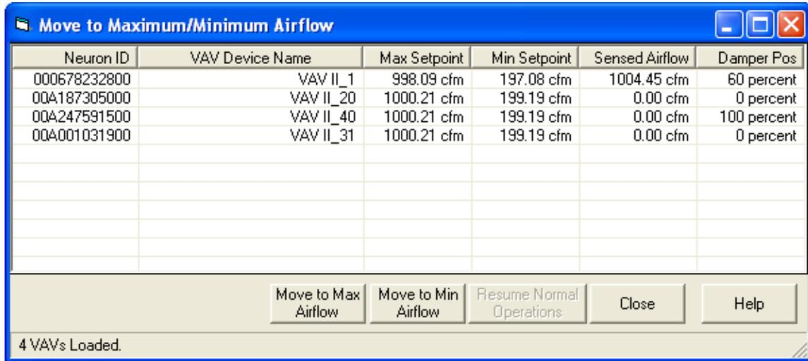
Fig. 13. Move to Maximum/Minimum Airflow.
